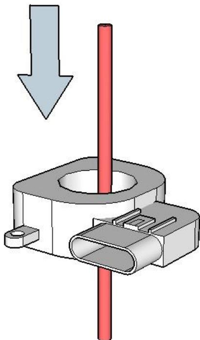
For even more accurate measurements up to 125 ampere, put the cable four times through the current sensor hole. Wire as the following picture.
