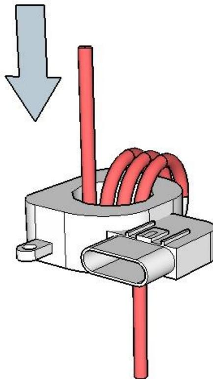
For even more accurate measurements up to 250A, put the cable twice through the current sensor hole. Wire as the following picture.
