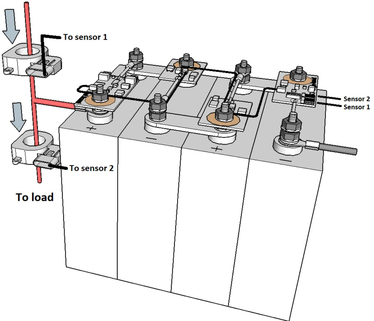
For current measurements up to 500 ampere, wire as the following picture.
